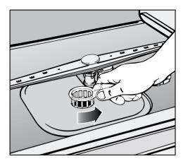
■ Turn the handle counterclockwise to release the filters.
